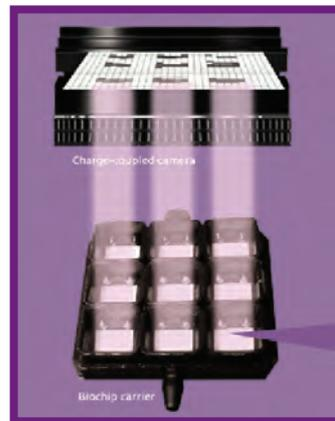
2. The CCD Camera is made up of a collection of light sensitive diodes which convert light into electrons to produce an electrical charge. The brighter the light that hits a single diode, the greater the electrical charge that will accumulate at that site.
