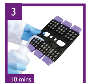
Wash biochips - 2 quick washes, 4 soaks for 2 minutes each
